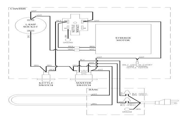
Fig. 2 Circuit Diagram Wiring of a Pop-Corn Machine
